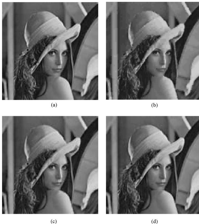
Fig. 4. LENA image and its reconstructed images with 64 codewords: (a) original image; (b) LBG; (c) DCT + LBG (VQ); and (d) DCT + CFPCM (VQ).
